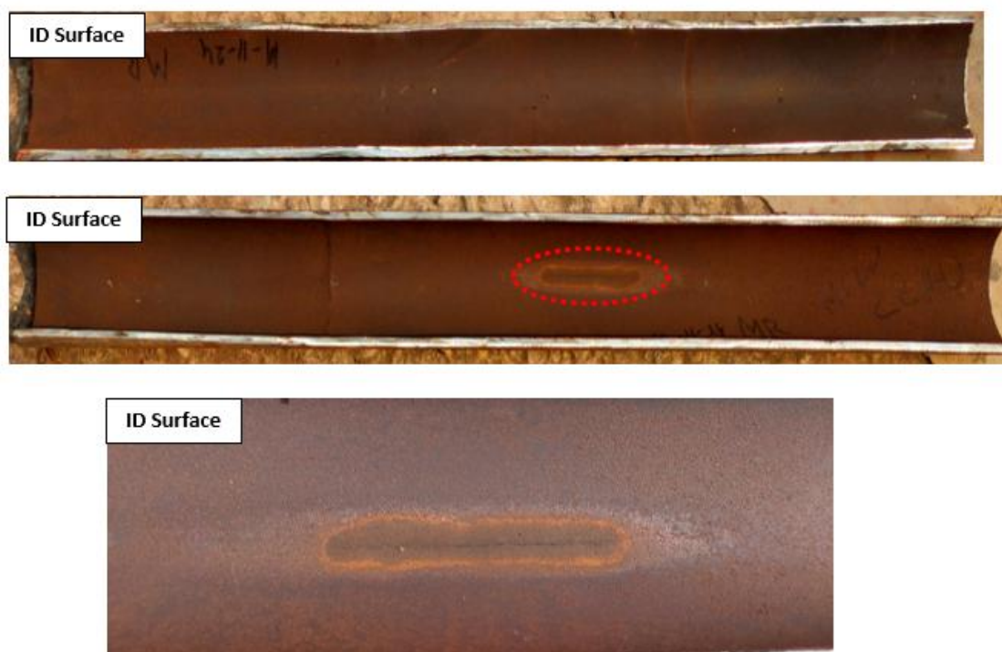
Fig. 7-9: ID Surface devoid of Fine longitudinal cracks except one major crack at the leaked location
