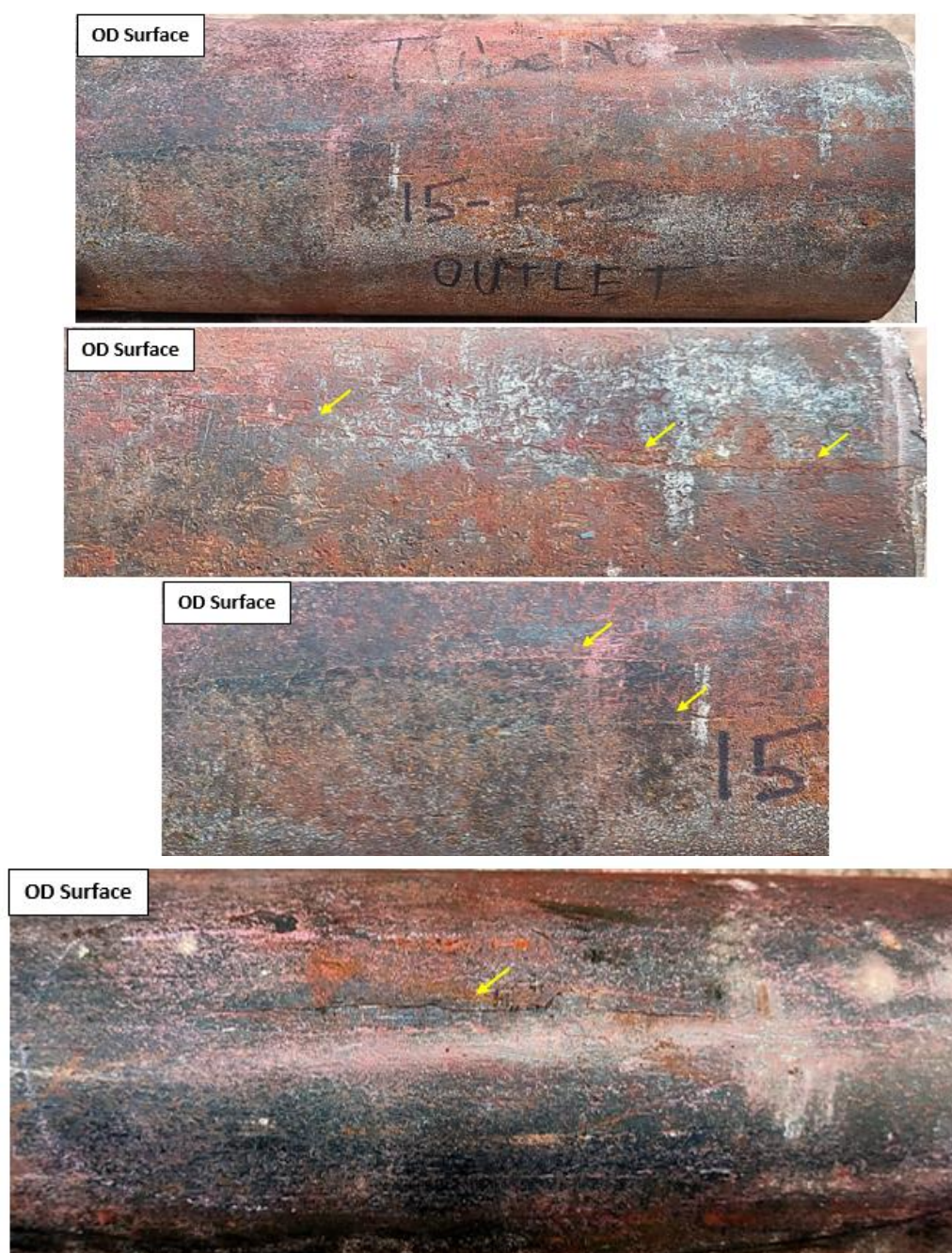
Figs.2-6: Multiple Fine longitudinal cracks at the OD surface of the tube
