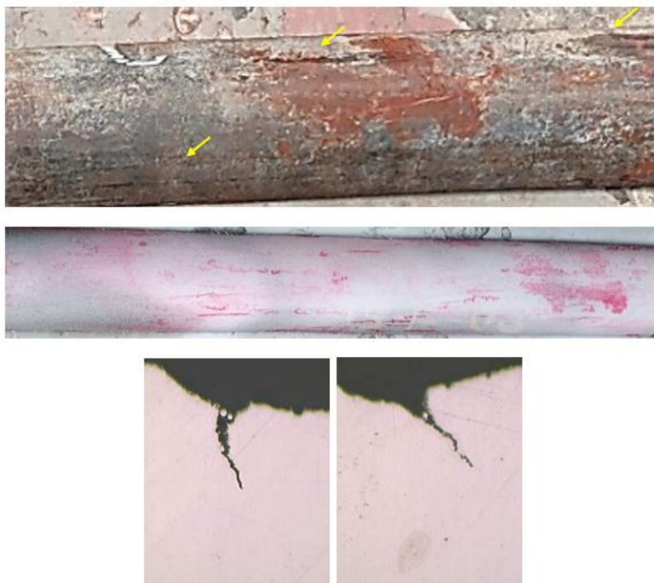
Fig.29-32: A Typical appearance of lamination defect in the seamless tube
