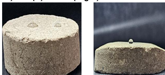
Figure 3.1. (A) Carbonate cores water wet (Left) and (B) oil wet (Right).
