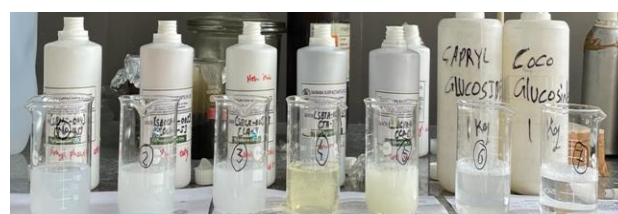
Figure 3.7. Non-ionic surfactants used for wettability alteration on calcite
