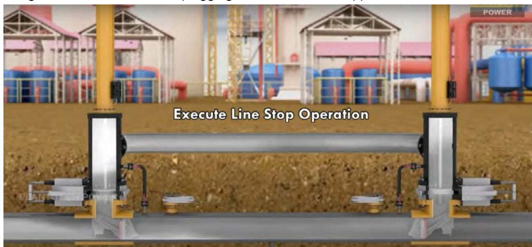
Fig 1: Representative schematic of "Line stop" Operation
