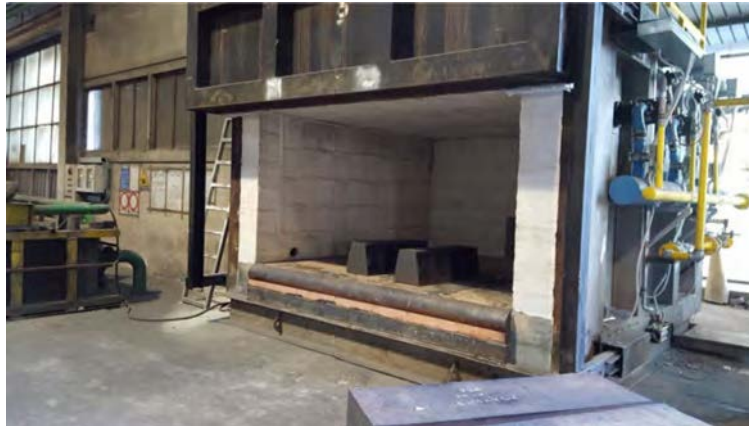
Figure 5: FAV industrial furnace selected for the H 2 NG trial
